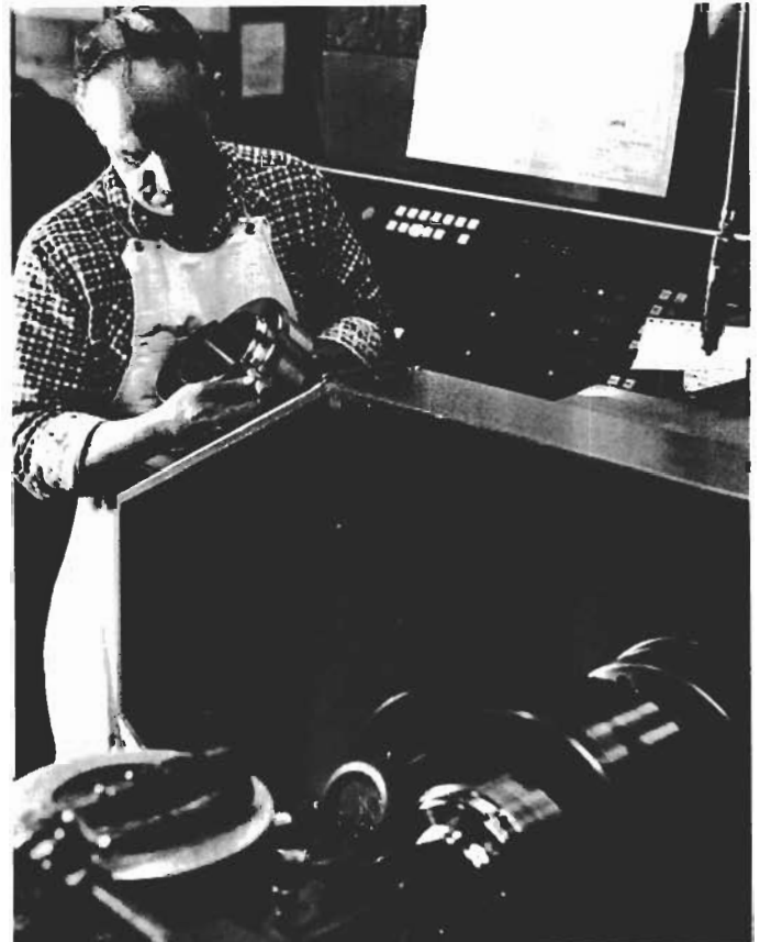
The operator of a numerically controlled lathe inspects a part to see if it is within tolerance. Since the use of N/C machine tools eliminates human error, occasional spot checking for out-of-tolerance measurements due to tool wear is all that is needed.
