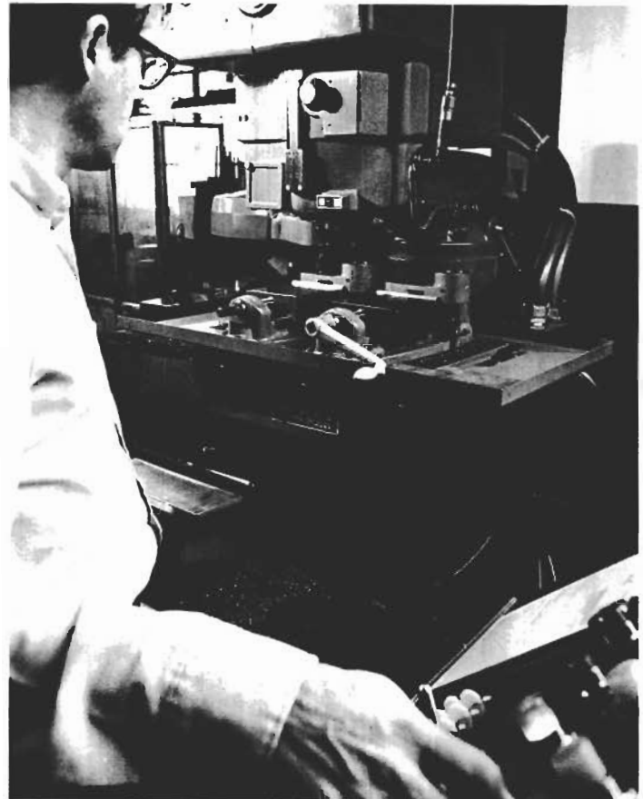
Tapes are edited and verified on the 9820 instead of tying up an expensive N/C machine tool such as this 3-axis machining center at Buerk.
