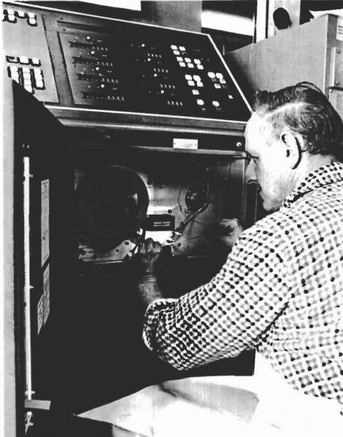
The finalized tape is loaded into the controller for an N/C machine.
