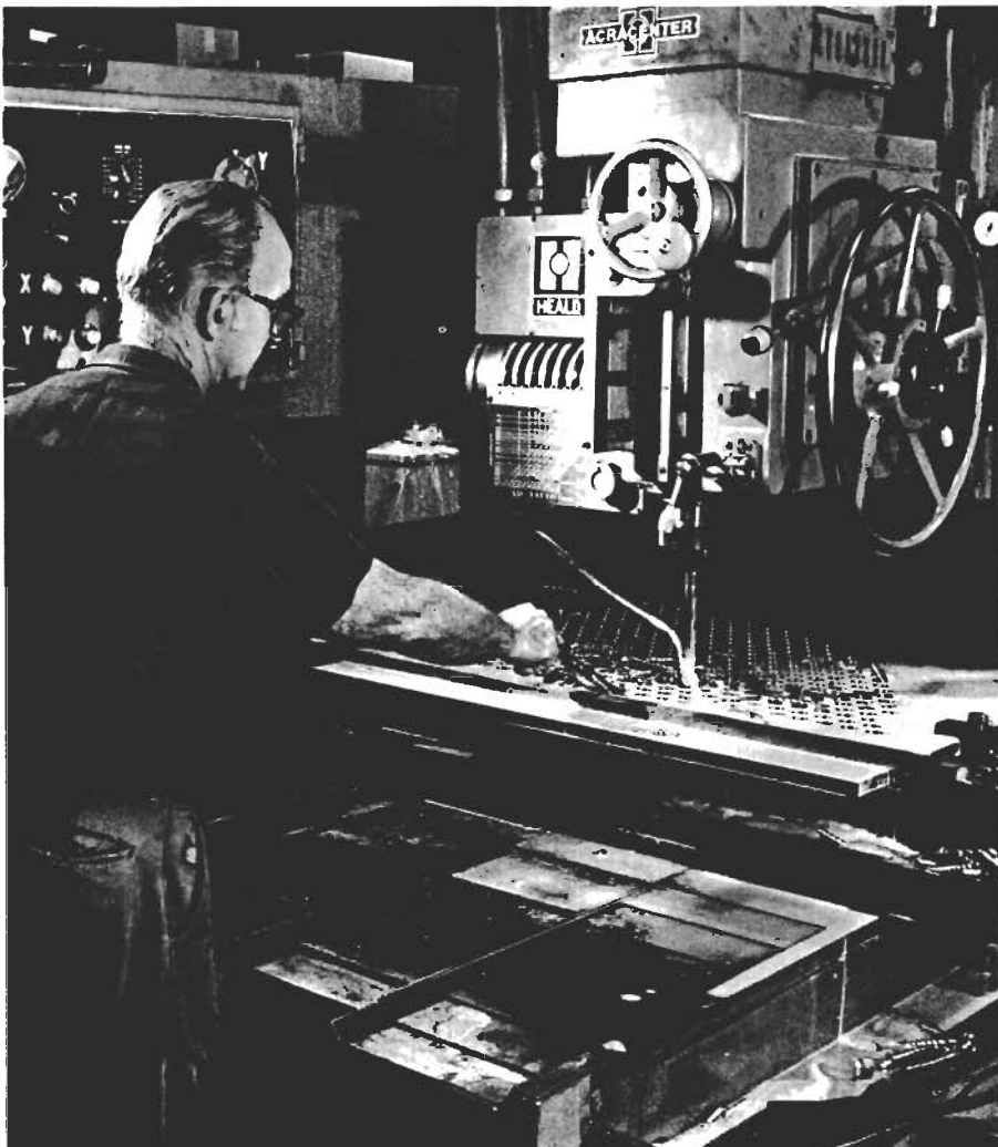
This N/C 2-axis machining center is drilling a template for a larger production part.
